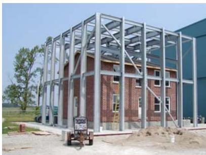
Figure 1: Full-scale house test specimen inside galvanized steel reaction frame.
