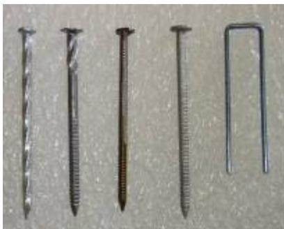
Photograph of the different nails used in the roof sheathing study. From left to right: twist-shank nail, HurriQuake® nail, adhesive coated ring-shank nail, another ring-shank nail, and a staple.
