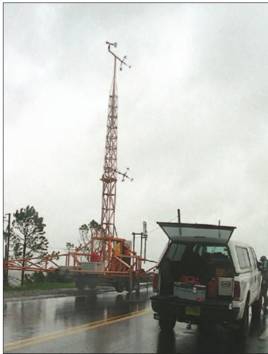
**Researchers set up a 10-metre-high tower just hours prior to Hurricane Dennis making landfall. This tower measured a three-second gust speed of about 120 mph as Hurricane Dennis' eyewall passed over Navarre, Florida.**
