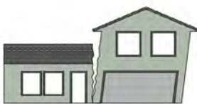
Home tears apart during earthquake.
