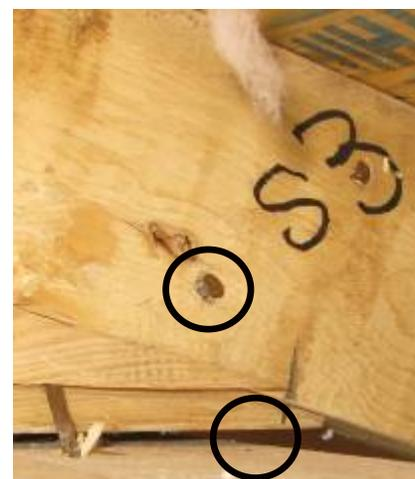
Figure 5: Roof connection after Dynamic Test #3. The nails moved considerably, and a large gap appeared between the joists and trusses.
